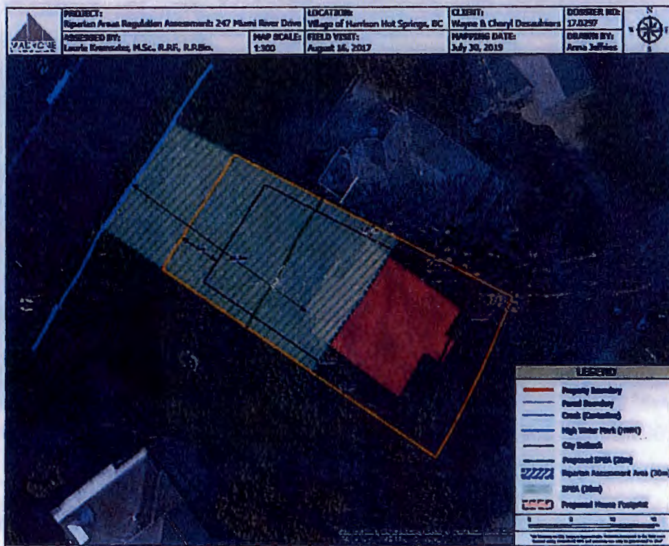
Figure 5: Proposed house footprint and requested variance of SPEA to 20 m. Note deck is at 25 m and house outside of the hardship SPEA of 28.4 m.
