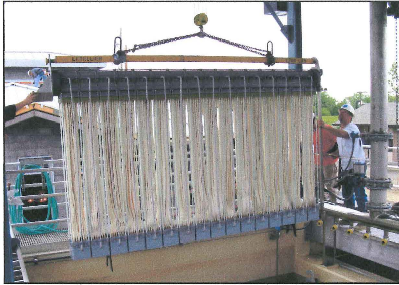
Figure 4: Siemens rack assembly fitted with sixteen (16) membrane modules and supported by a rack lifting beam during removal from tank.
