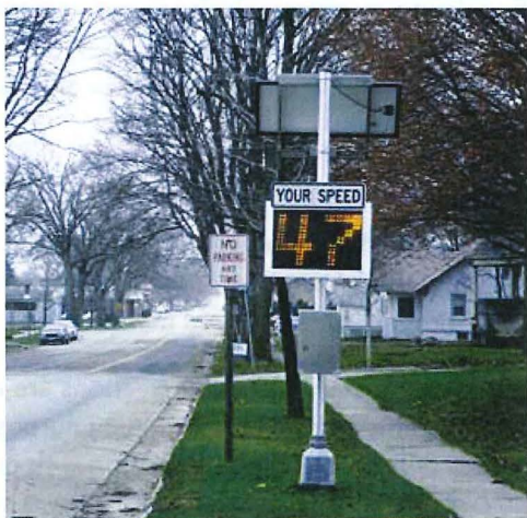
Figure 3.6: Example of Speed Feedback Signage
